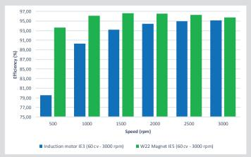
IE5 efficiency levels were calculated considering the IE4 levels with 20% lower losses.
